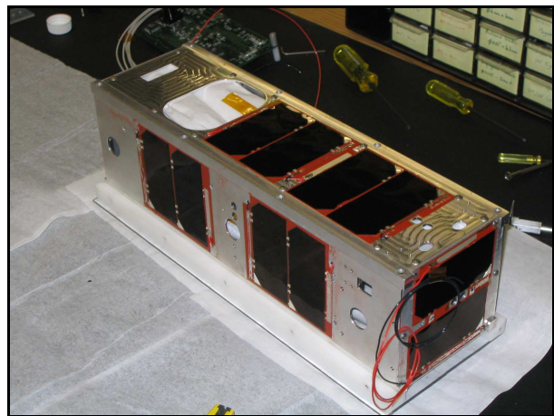
Figure 7 - Partly integrated CanX-2 spacecraft
