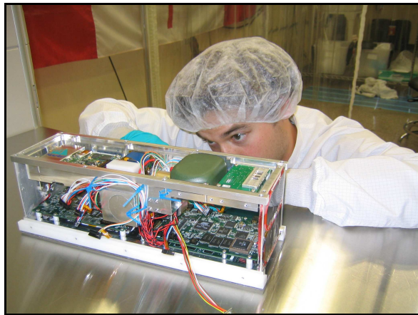
Figure 1 – CanX-2 being assembled by a Masters student in the SFL clean room.
