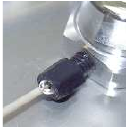
Figure 2: Propellant Leakage Occurring Through a Ferruled Connection with PEEK Tubing
