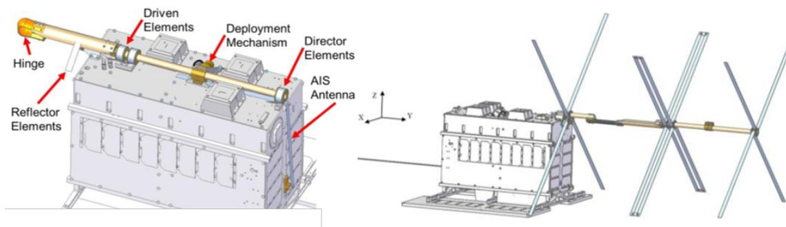
Figure 7: Deployable Yagi Antenna
