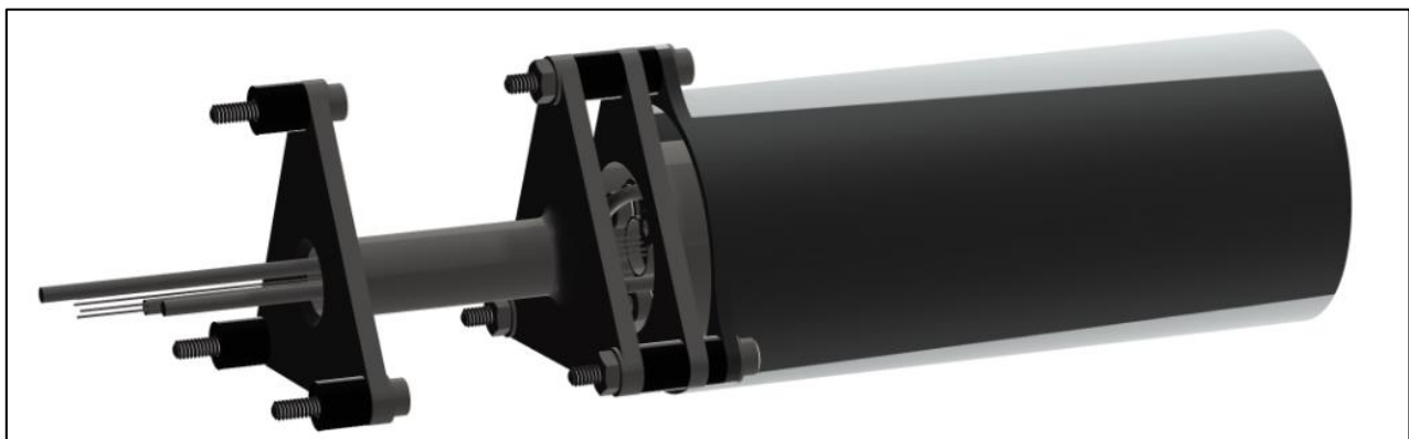
Figure 3: CAD model of the nitrous oxide monopropellant thruster prototype.
