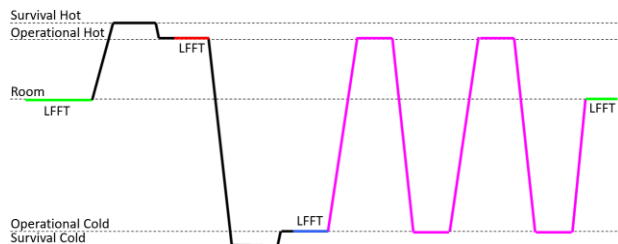
Figure 18: Temperature Profile for Magnetorquer Thermal Cycling Testing
