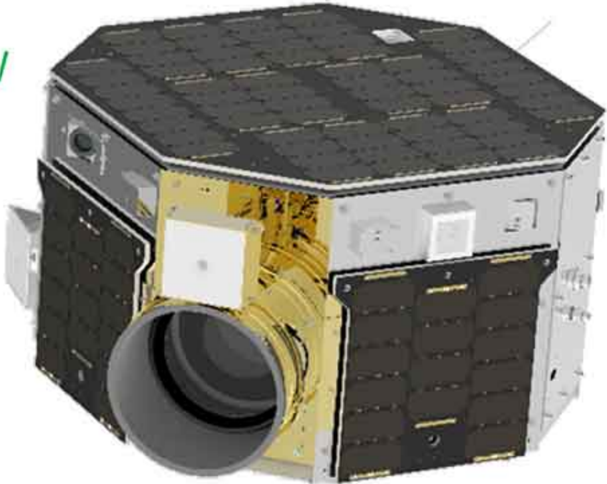
NAUTILUS – up to 150 kg 60 x 60 x 60 cm, scalable Payload: up to 90 kg, 525 W
