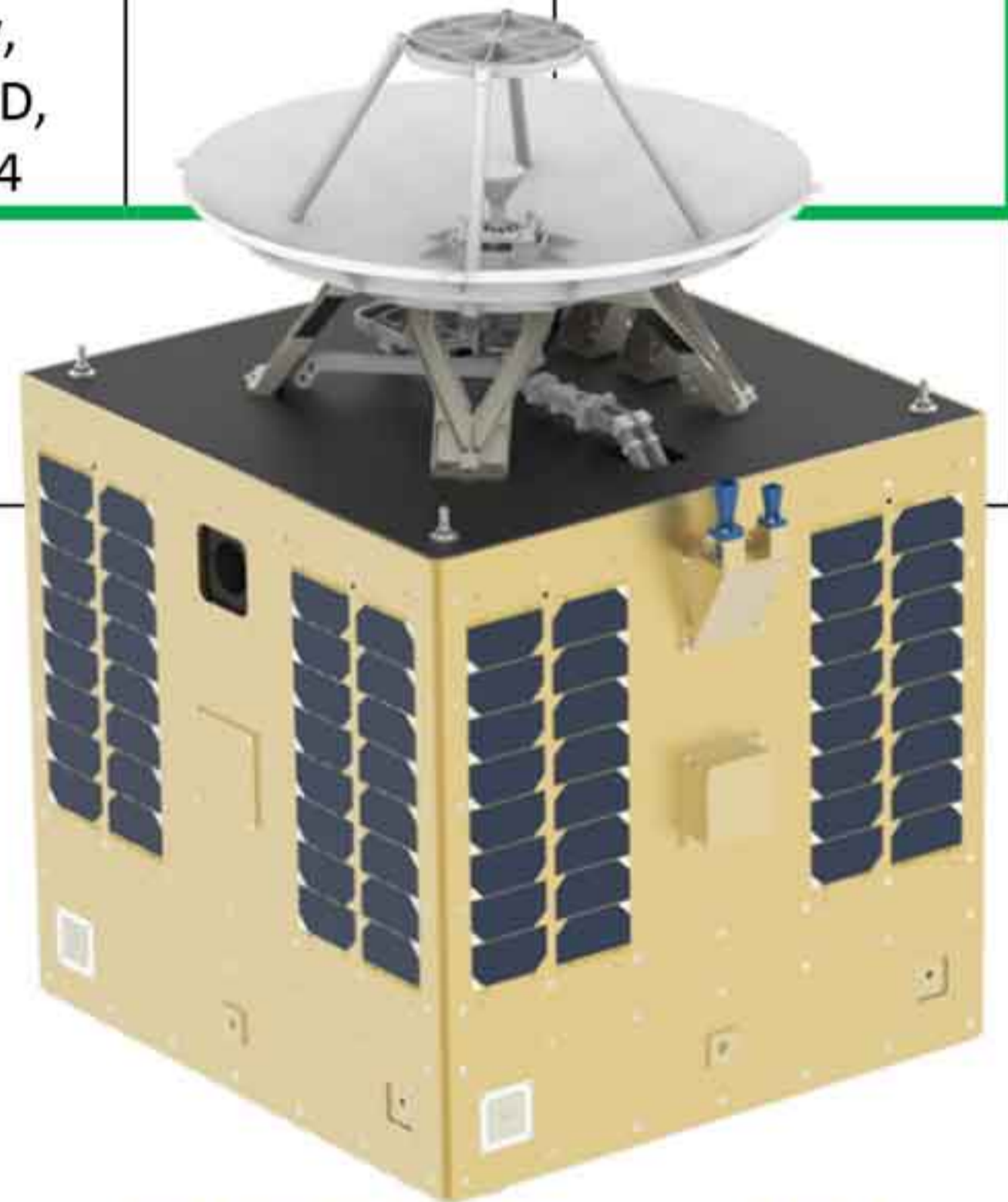
DAUNTLESS – up to 500 kg 1 x 1 x 1 m, scalable Payload: up to 300 kg, 800 W
